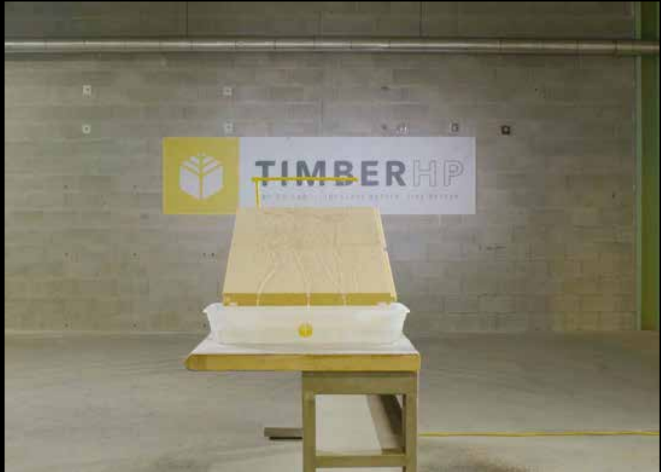
Bulk moisture demonstration
