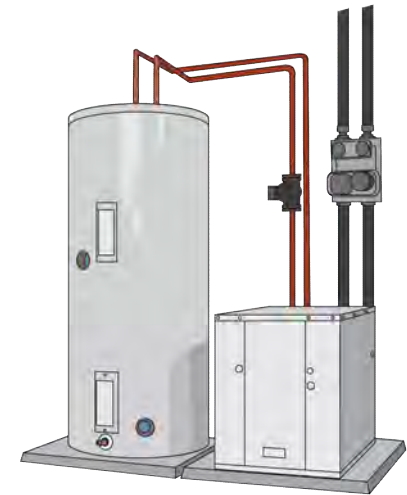
Ground-Source Heat Pumps (GSHP)
