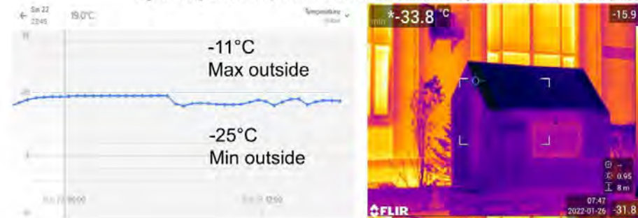
Fig.6 Hourly indoor temperature and thermal camera image of the Goldfish house project
